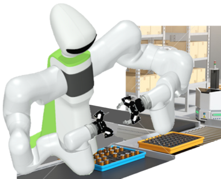
A Dual Arm Collaborative Robot in Industrial Applications
