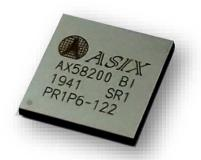
The AX58200 is a 2/3-port EtherCAT Slave Controller SoC equipped with ARM® Cortex®-M4F core with DSP extension runs up to 192 MHz and EtherCAT Slave Controller (ESC) with two integrated Fast Ethernet PHYs. AX58200 also supports additional communication interfaces such as 10/100Mbps Ethernet MAC with RMII and hardware cryptography accelerator, HS USB OTG, SPI/UART/I2C/I2S/CAN/PWM, etc.
