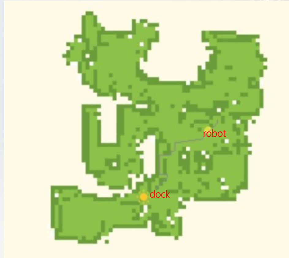
M660GMA 2 Gyro + encoder inertial mapping
